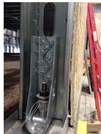
Figure 5. Left: Phase 1 building at peak drift, with plots of hold down forces. Clustered hold down forces (all red, for example), indicate Type 2 behavior. Right: photograph of load cell installed in shear wall hold down.
