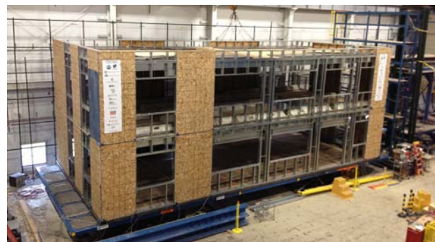
Figure 1. At left, engineering drawing of the LRFS and gravity system, at right, the Phase 1 building as built and tested.
