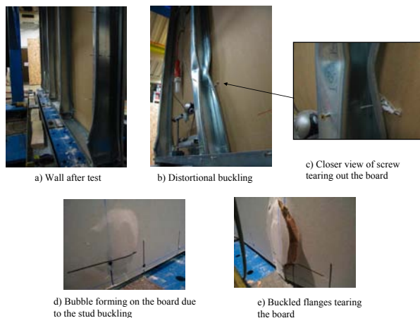
Figure 3: Response of gypsum sheathed walls [3]
